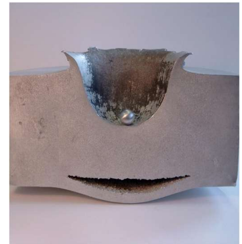
12.7mm diameter impactor, 90mm Al target, 6.8 km/sec impact velocity. (Image courtesy ESA).
